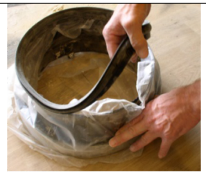
4. Remove the gasket and discard the Longopac rest
