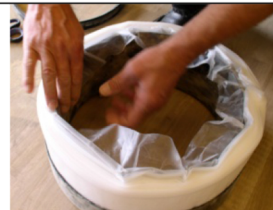
7. Fold the inner Longopac over the edge
